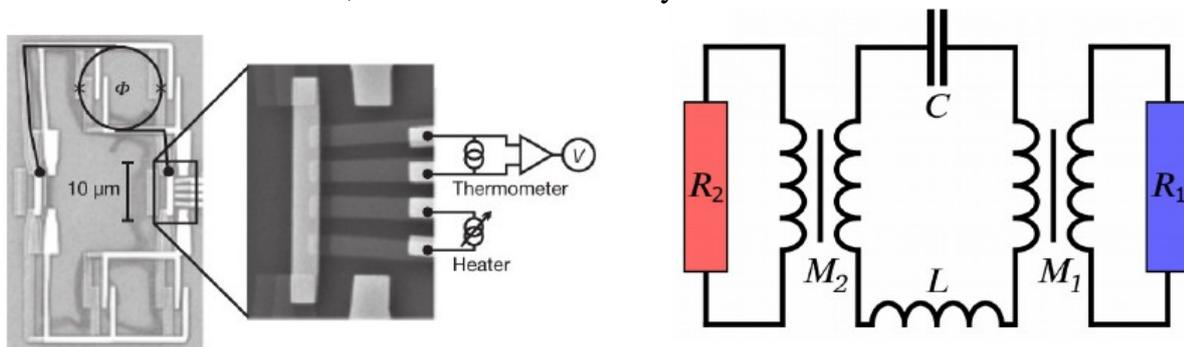
This system can be modeled by an effective electric circuit (right figure), where the metallic islands are represented by resistors  $R_1$ ,  $R_2$ , the superconducting resonator by an  $LC$  contour, coupled to each other by mutual inductances  $M_1$ ,  $M_2$ . Average heat current in this circuit has been calculated using the semiclassical approach of fluctuating electrodynamics [2].
