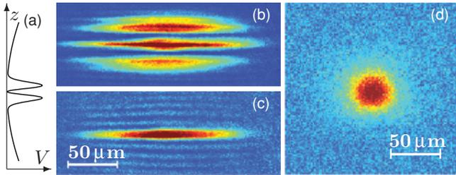
FIG. 1. (Color online) (a) Potential  $V$  along the vertical direction  $z$  produced by the magnetic trap and the laser beam. (b,c) Side view of the cloud before (b) and after (c) depumping atoms in the side wells. The horizontal stripes are due to diffraction. (d) Top-view *in situ* image yielding fit parameters  $T = 132$  nK and  $\alpha = 0.29$  (for  $\xi = 0.25$ ).
