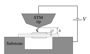
Figure 2.1: Schematic drawing of a carbon nanotube suspended over a trench. A bias voltage is applied between the STM tip (source) and substrate (drain). The inflated portion in the suspended portion of the nanotube illustrates the radial breathing mode. h is the tip-nanotube separation at rest.
