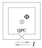
**Figure 5.2:** Sketch of the Andreev level qubit: a low inductance superconducting loop with a quantum point contact (QPC).  $\Phi$  is the magnetic flux; the arrows indicate fluctuating persistent currents.
